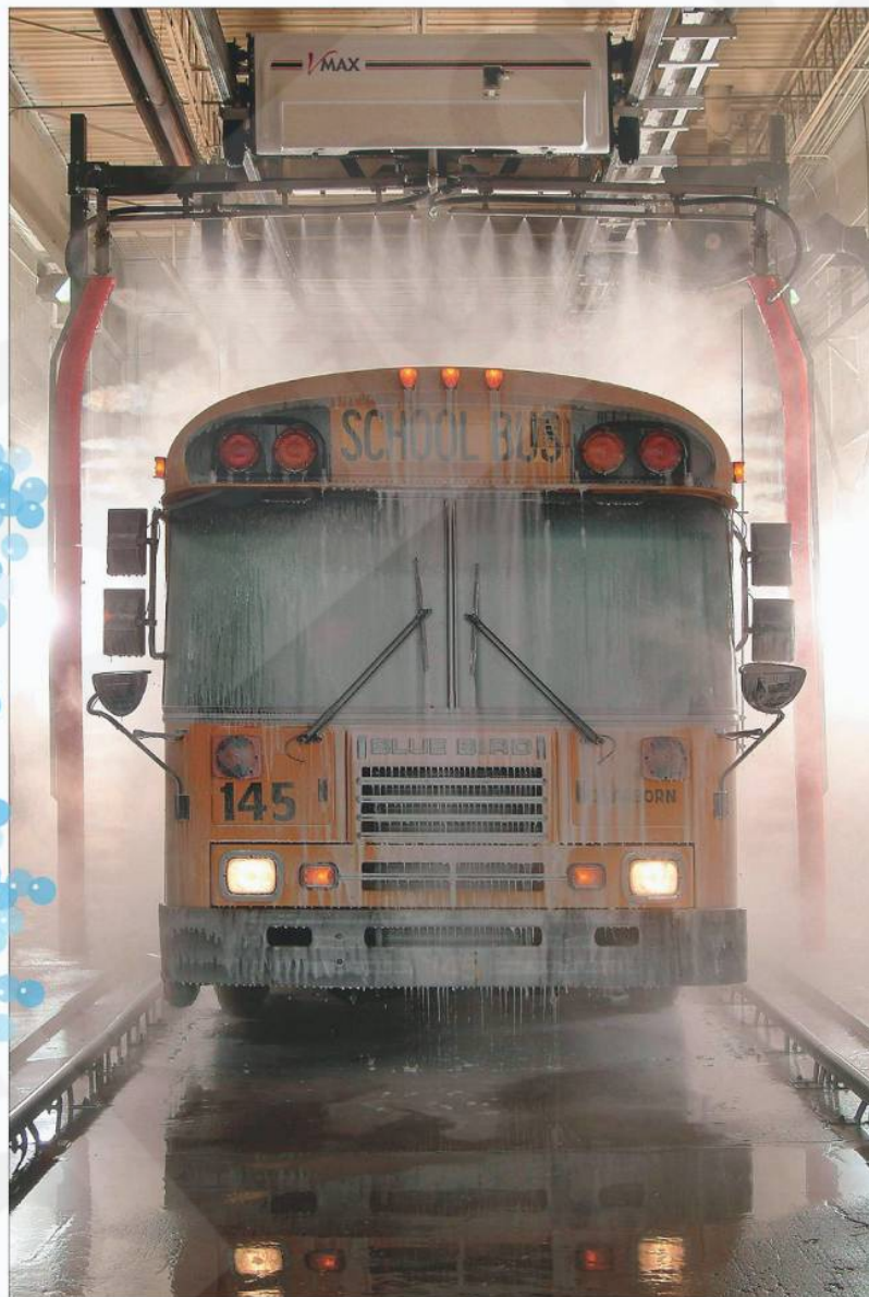
Belanger's V-Max touchless wash system uses high-pressure water rather than brushes to clean vehicles.
