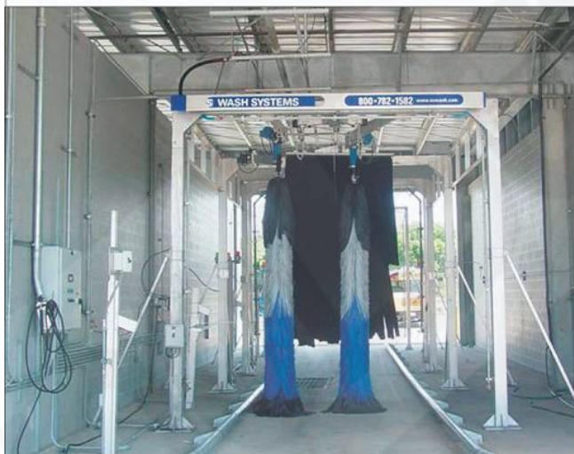
The 3100 drive-through wash system from NS Wash Systems features a scrubber curtain that cleans the hood and top of a bus, as well as two vertical brushes for the sides and back.
