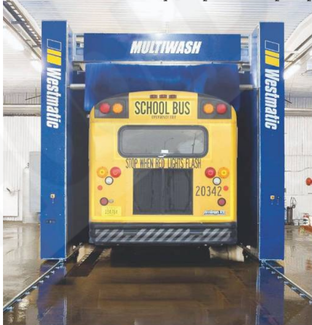
Westmatic Corp.'s Multiwash system includes programmable logic controller technology that monitors and adjusts brush pressures to provide a consistent wash.
