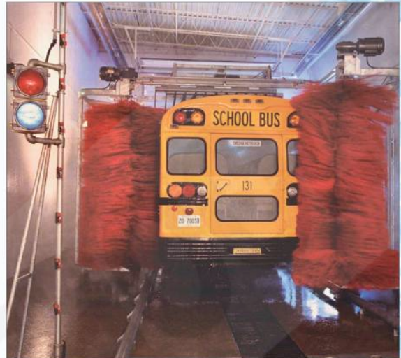
Ross & White Co.'s Hybrid System consists of two vertical brushes that clean the sides and rear of the vehicle, and touchless water pressure to clean the more fragile hood and mirror areas.
